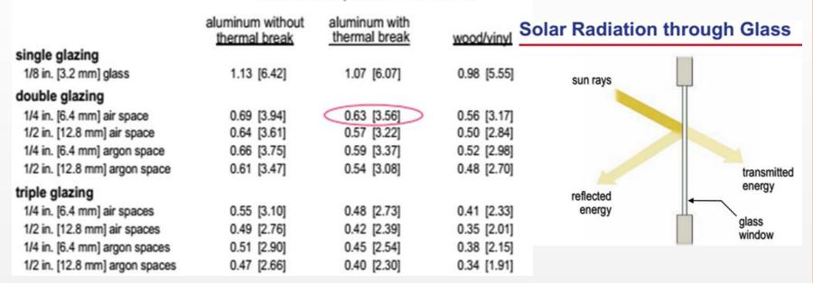
The windows in our example are double-pane windows with a ¼-inch [6.4 mm] air space between the panes. Assuming that the windows are fixed (not operable), with aluminum frames and a thermal break, the U-factor is 0.63 Btu/hr • ft² • °F [3.56 W/m² • °K].
